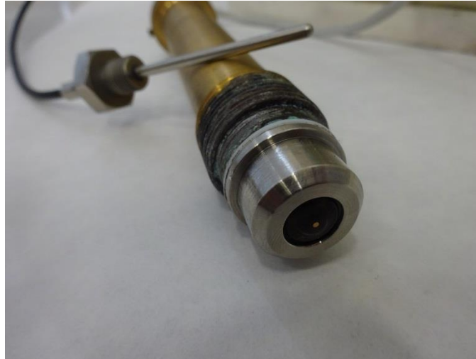
Figure 4: hydrogen sensor - detailed view of the membrane covered anode and thermometer
