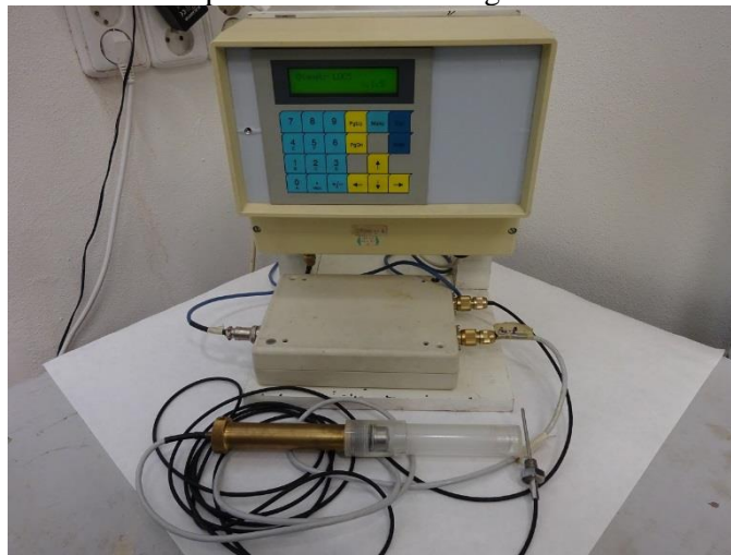
Figure 3: 1990's measurement device to measure oxygen and hydrogen concentration
