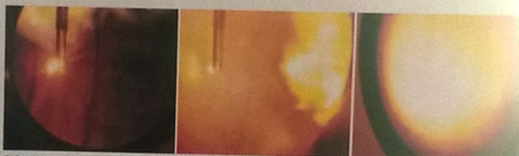
FIGURE 2 Development of the flames (10.0 vol.% COG, 90.0 vol.% of air) in the course of an explosion
