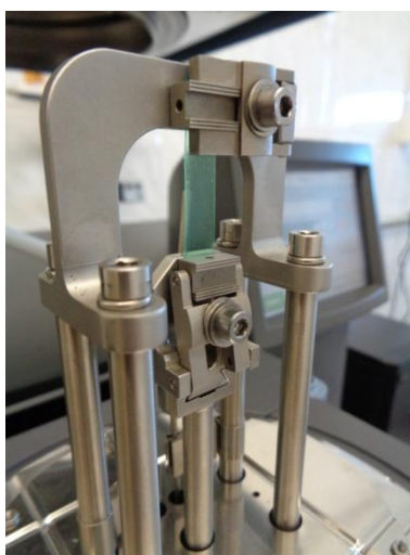
Fig.2 Geometry tension - film for DMA analysis
