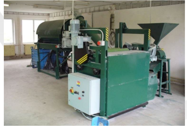
Line for crushing windscreens [source: www.maveba.eu ]
