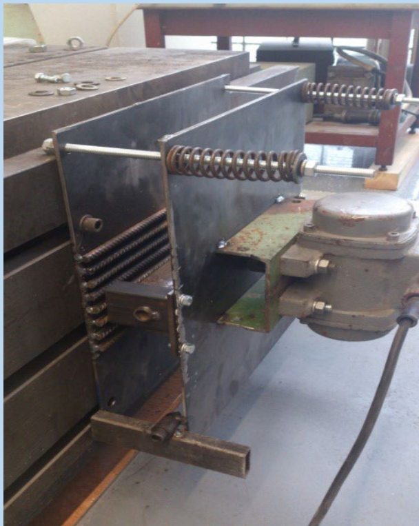
Laboratory model of vibration wrapping glass from foil
