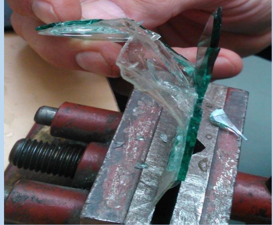
Separation of foil from glass by heating
