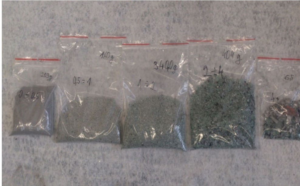
Individual batches of glass sample 1 after sieve test
